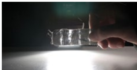
Filter fabric 10µm ( mesh 660/63 ) before cleaning
