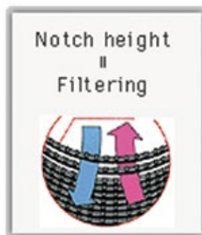
Filtering principle of the notch wire filter elements
