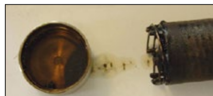
So we found the filter candle, cap- and end piece partly loose.
