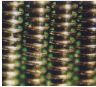
Same filter tissue 10 µm, cleaned
