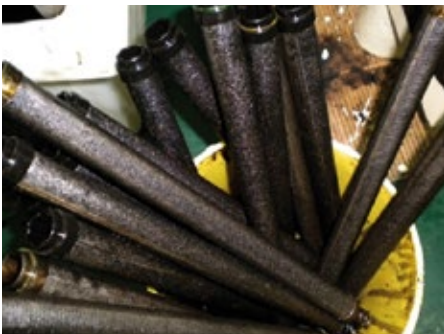
Candle filter before cleaning in ultrasonic bath
