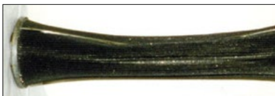
Here we have a sample of saucer eyed weld
