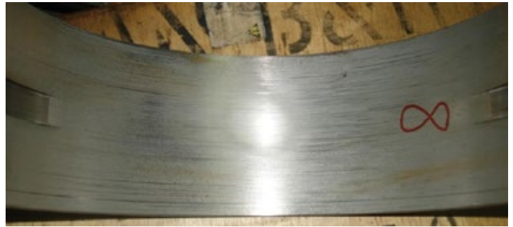
Bearings after a running time of 15,000 hours
