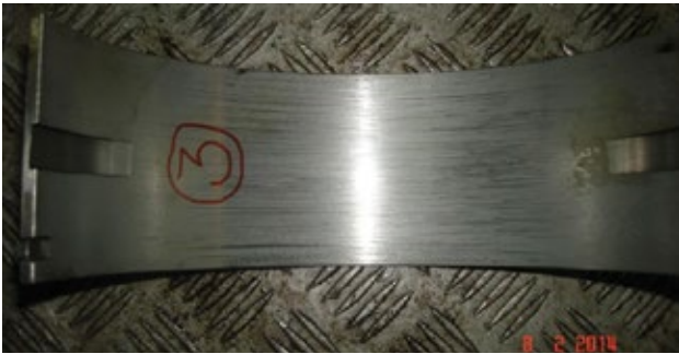
Bearings after a running time of 15,000 hours
